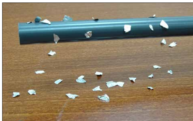
Figure 38. Electrified PVC bar attracting little aluminium pieces.
