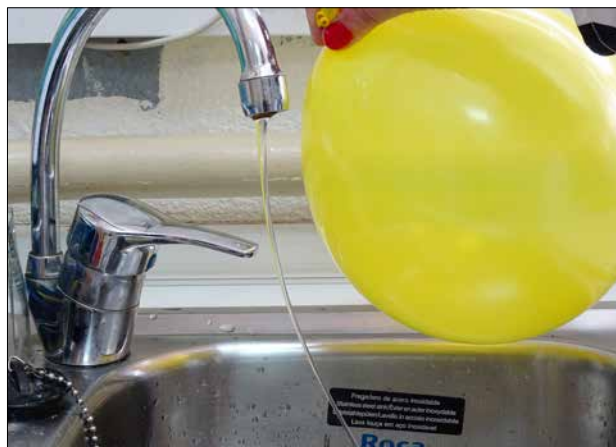
Figure 35. An electrified balloon attracts a narrow stream of water.
