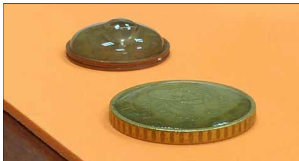
Figure 32. Cohesion between water molecules; adhesion between the molecules in water and the coin.
